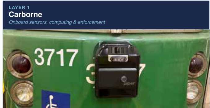
Front sensor assembly — UWB Sensor and TrackSight™ LiDAR on the front of a light rail vehicle.
