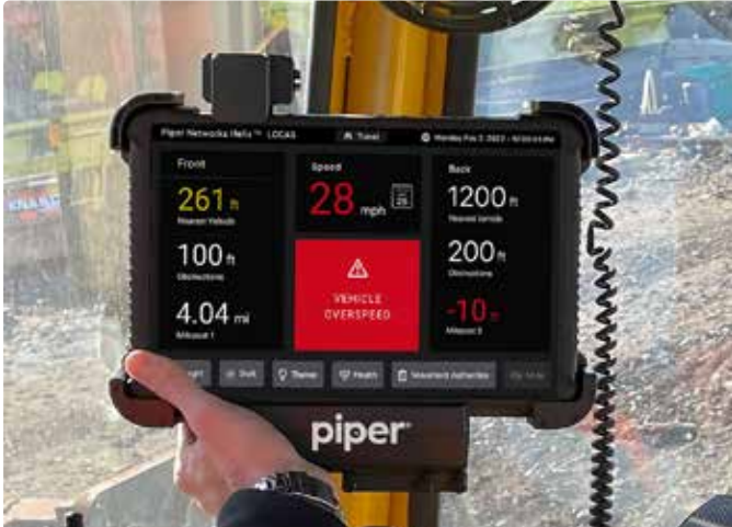
Piper Train Operator Display — Real-time collision avoidance and warnings delivered to the operator.
