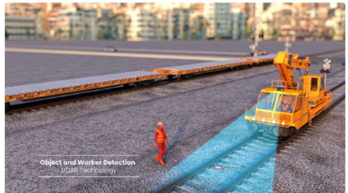
Object and Worker Detection — TrackSight™ LiDAR scanning the fouling envelope ahead.
