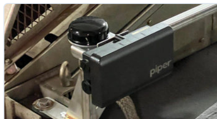
Carborne installation — UWB tag and GPS antenna are easily mounted on the roof of the vehicles. No undercarriage work required.
